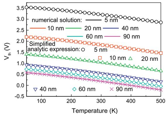
**Fig. 2.** The threshold voltage as a function of temperature with grain-boundary acceptor trap density of  $1.0 \times 10^{11} \text{ cm}^{-2}$  and the active dopant density of  $1.0 \times 10^{14} \text{ cm}^{-3}$ .
