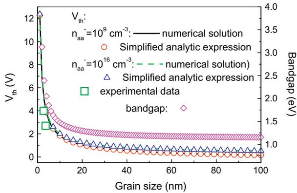
**Fig. 3.** The threshold voltage as a function of the size of silicon grain with grain-boundary acceptor trap density of  $1.0 \times 10^{11} \text{ cm}^{-2}$  under temperature of 300 K for different the active dopant density. The band gap as a function of the size of silicon grain is also given.
