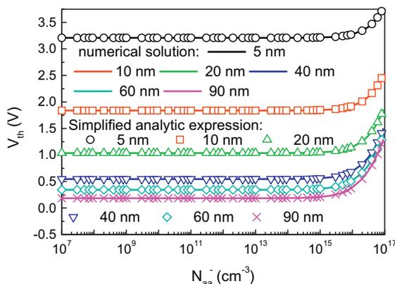
**Fig. 4.** The threshold voltage as a function of the active dopant density with grain-boundary acceptor trap density of  $1.0 \times 10^{11} \text{ cm}^{-2}$  under temperature of 300 K for different values of the size of silicon grain.
