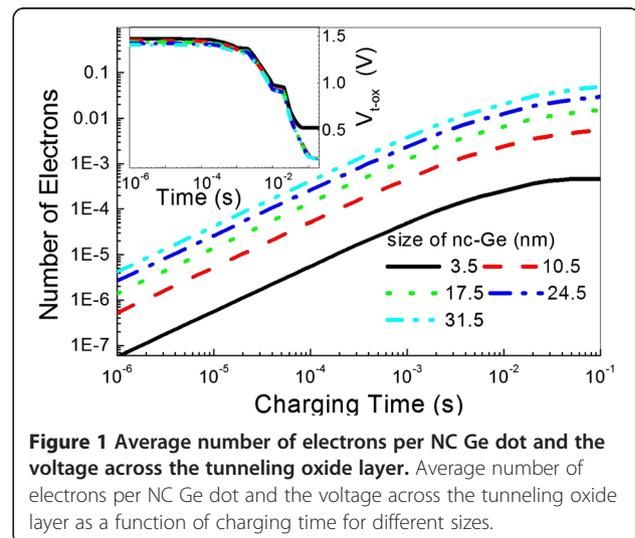
**Figure 1** Average number of electrons per NC Ge dot and the voltage across the tunneling oxide layer. Average number of electrons per NC Ge dot and the voltage across the tunneling oxide layer as a function of charging time for different sizes.
